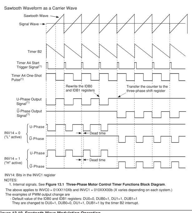
Figure 13.10 Sawtooth Wave Modulation Operation
